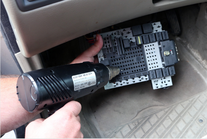
Fig. 1 Use a hair dryer or electric heat gun to heat up the CEM for 5 minutes.
